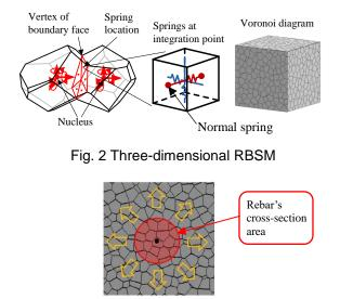
Fig. 4 Corrosion expansion model
