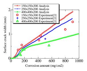
Fig. 20 Surface crack width propagation in cases of various sizes specimens
