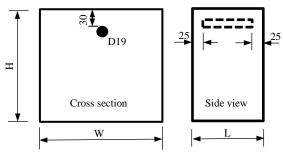
Fig. 18 Specimen set-up (various sizes)
