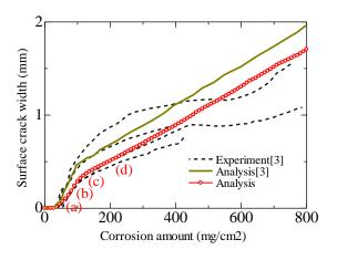
Fig. 13 Surface crack width propagation
